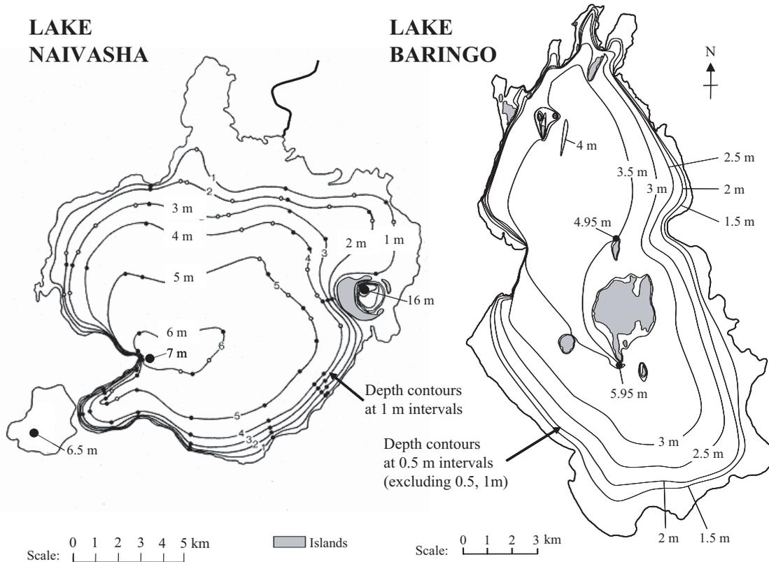
**Fig. 1.** Bathymetric maps for Lake Naivasha (August 1991; after Hickley *et al.* 2002) and Lake Baringo (August 2003). Contour lines are 1 m and 0.5 m (commencing at 1.5 m) intervals respectively. Spot depths for deepest points shown; contour lines <3m around Baringo islands not shown.
